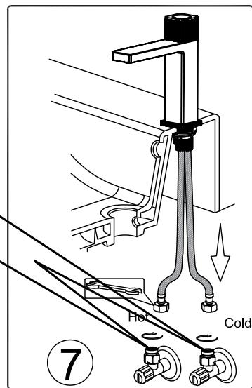
7. Install the Check valve connector(9) to angle valves linked with Hot & Cold water supply pipe, then fasten it by spanner to the other end of the Hot & Cold Inlet flexible hose(5).
