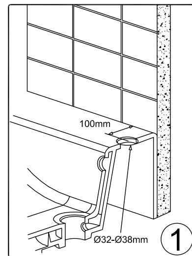
1. Make a hole on the counter at  $\Phi 32$  -  $\Phi 38$ mm
