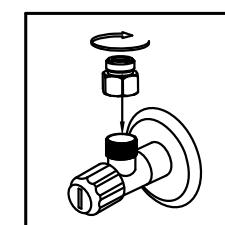
MAKE SURE the Check valve connector is installed to the angle valve first before the angle valves connect with the Inlet flexible hose.
